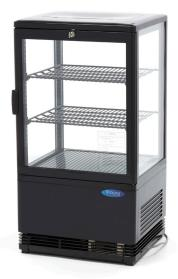
Beautiful refrigerated black showcase 58L Painted steel with plastic Double glazing on 4 sides Equipped with 2 coated grids Cooling with fan Automatic defrosting Refrigerant R290 / CFC-free Dixell digital temperature controller Temperature 0°C to 12°C Door with lock LED lights inside Fixed feet
