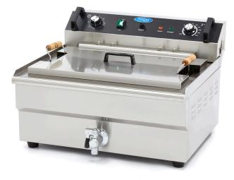
Deluxe single tank fryer Complete with oil valve Very nice finishing Completely made of stainless steel Detachable lid With cold zone Protected heating elements Adjustable thermostat: 0°C to 200°C Overload protection Stands on four rubber feet Tank capacity: 38.5 liters Min. oil quantity: 17 Liters Max. oil quantity: 30 Liters
