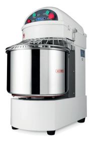
Professional spiral mixer Dough kneader with very strong motor With drive chain and v-belts Metal housing with durable coating Axle and spiral made of stainless steel Protective metal guard With safety switch Stands on four rubber feet Easy to clean Spiral speeds: 110 & 240 RPM Bowl speeds: 10 & 20 RPM
