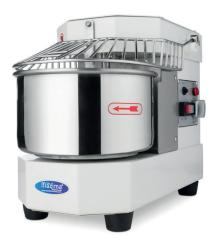
Professional spiral mixer Dough kneader with very strong motor Driven by v-belts Metal housing with durable coating Bowl can not be removed Protective metal guard With safety switch Stands on four rubber feet Easy to clean Spiral speed: 159RPM Mixing bowl speed: 21RPM Max. quantity of flour: 3kg Max. quantity of dough: 4,5kg Min. quantity of dough: 1,5kg
